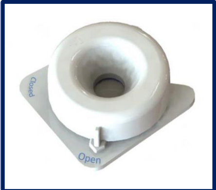
Cartridge Containing the electrode. CLOSED- OPEN- CLOSED position Dropper Containing the readout reagent
